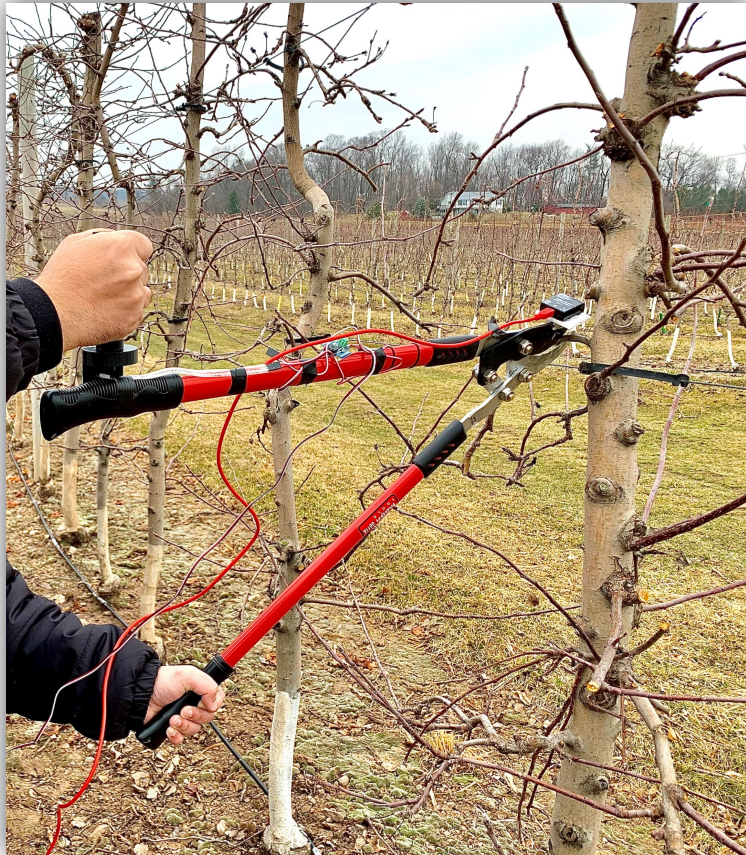
Cutting force and orientation measurement
