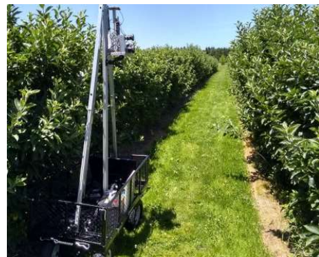
Figure 1. An image acquisition prototype using a wagon as a sensing platform. The wagon was equipped with a stereo vision camera to capture images of an entire canopy in 3D up to 14 ft.
