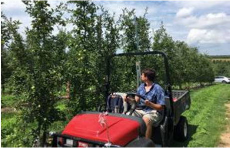
Figure 1. An image acquisition prototype using a ground vehicle as a sensing platform. The platform was equipped with multiple cameras to capture images of an entire canopy.
