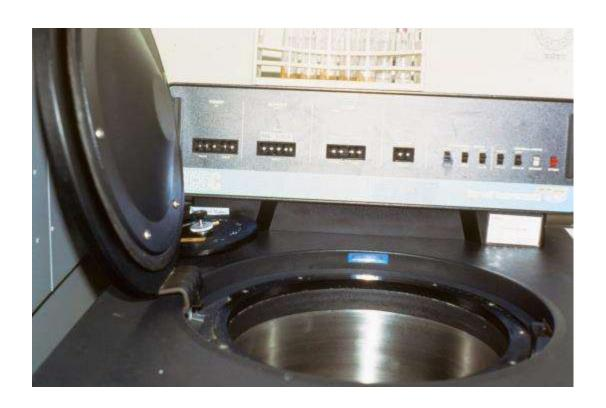
Centrifuge flesh to separate solid material from juice. Measure the weight of juice and pellet separately.
