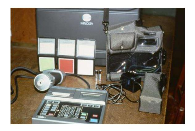
Fast electronic measurements measure light reflected from the fruit peel.
